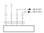
NM 230 A-F NM 24 A-F AC 19,2-28,8 V, 50/60 Hz AC 85-265 V, 50/60 Hz Power supply..... DC 19,2-28,8 V
