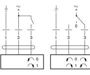
**GM 24 A** GM 230 A AC 19,2-28,8 V, 50/60 Hz AC 85-265 V, 50/60 Hz Power supply.....
